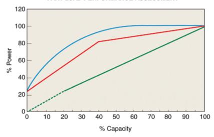
Single-Stage Lubricated Load/Unload
